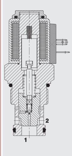
The directional valve is a pilot operated valve in poppet style.
