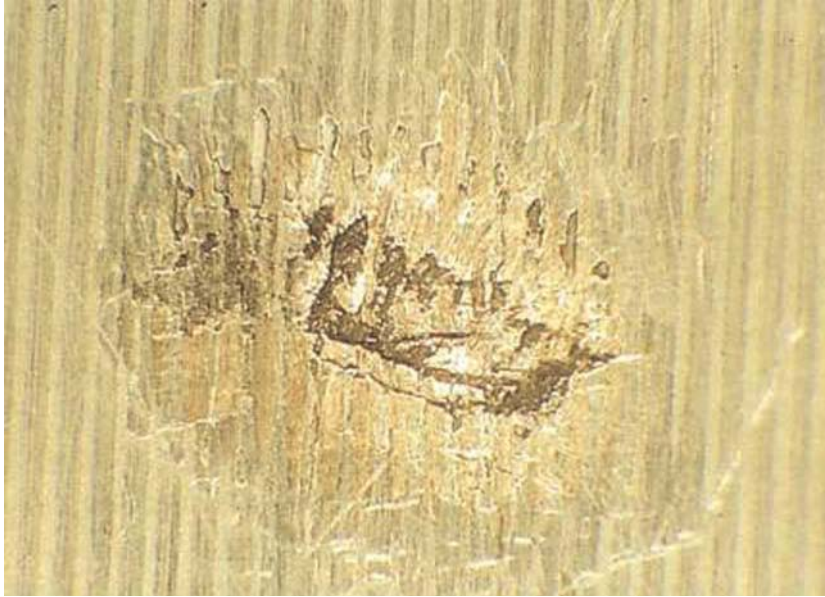
Fig. 8 Destroyed Raceway of a Ball Bearing Caused by Particulate Contamination
