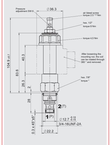
\*Torque: Steel manifold (ultimate tensile strength < 360 N/mm²): 35 Nm Aluminium manifold (ultimate tensile strength < 330 N/mm²): 30 Nm (tool acc. to DIN EN ISO 6789,
