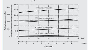
measured at v = 34 mm<sup>2</sup>/s,  $T_{oil} = 46$  °C
