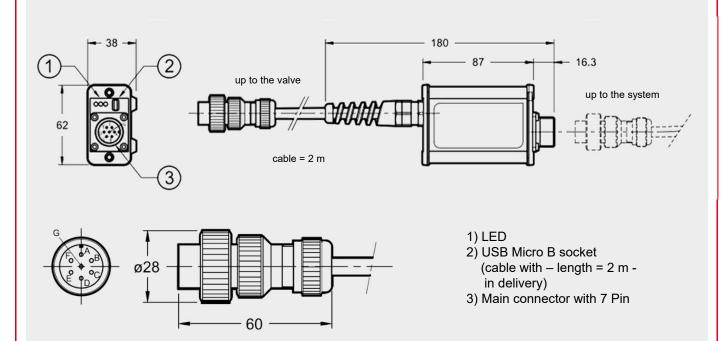
In the casing of electronics, a 7-pole port for connecting with external devices is integrated.
