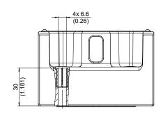
Fastening screws: (not included in scope of delivery) DIN EN ISO 4762 - M6 x 40 - 10.9 Tightening torque: 10 Nm
