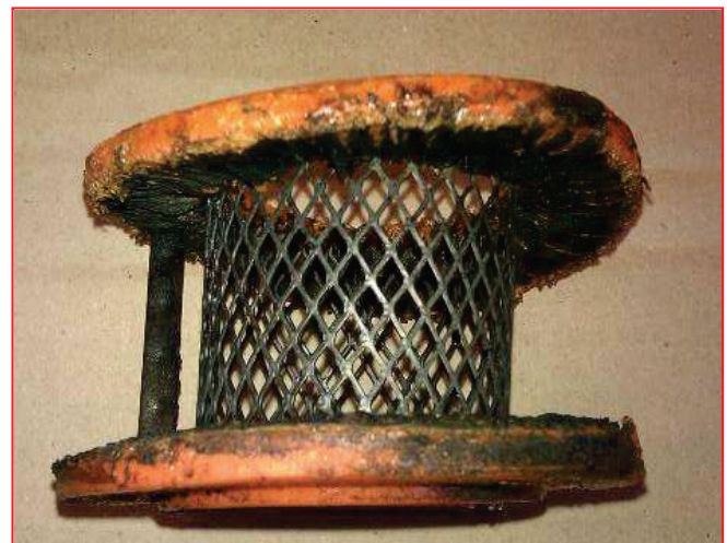
Breather filter burned as a result of explosion in the tank
