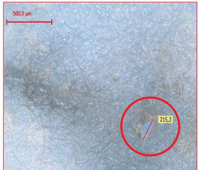
Burn hole in the filter material
