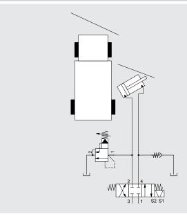
If the side plate meets an obstacle, the pressure in the cylinder line in front of DB12PK suddenly increases.
