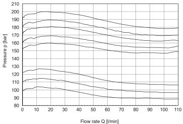
p/Q characteristic measured at  $v = 32 \text{ mm}^2/\text{s}$ ,  $T_{Oil} = 40 \text{ °C}$ Cracking pressure 40 / 55 / 65 / 75 / 90
