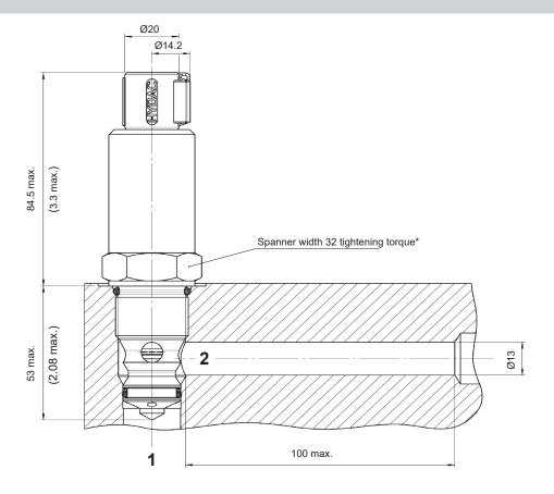
\* Tightening torque:
