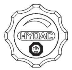
The symbol indicates the direction in which the pressure is changed when turned:
