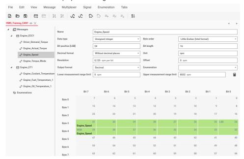
Signals and multiplexers are also visualised by a control element to support the user during creation/editing.
