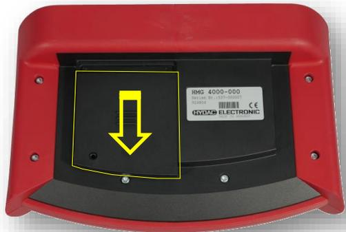
Loosen the connection plug of the battery pack.
