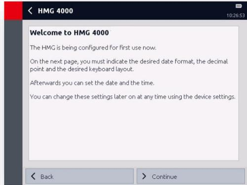
Select the desired date format, decimal point and keyboard layout. Complete the operation with "*Continue*" or go back to the previous screen by pressing "*Back*".
