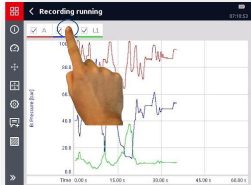
By ticking the corresponding selection box, you can show or hide each measurement channel separately in the graphic.
